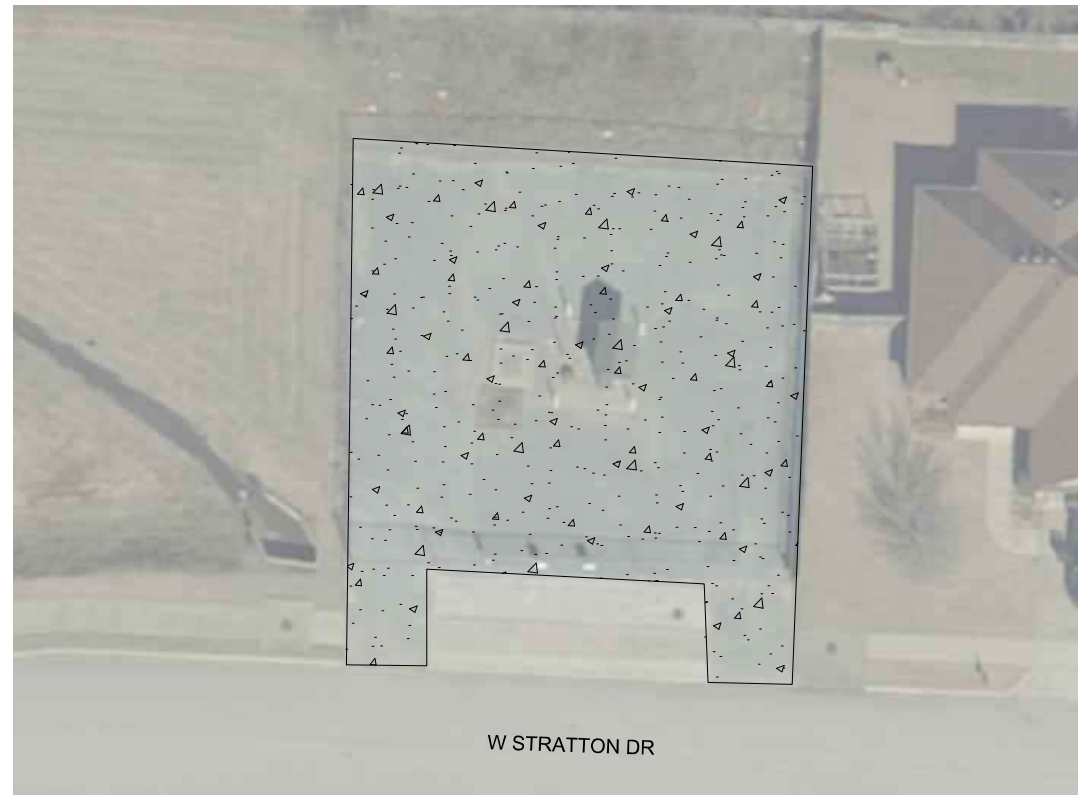
DIXIELAND LIFT STATION NTS Location: 1703 Stratton Rd, Rogers, AR 72756 Scope of Work: Crack Repair & Seal Coat Approx. Area: ~850 sq yd
