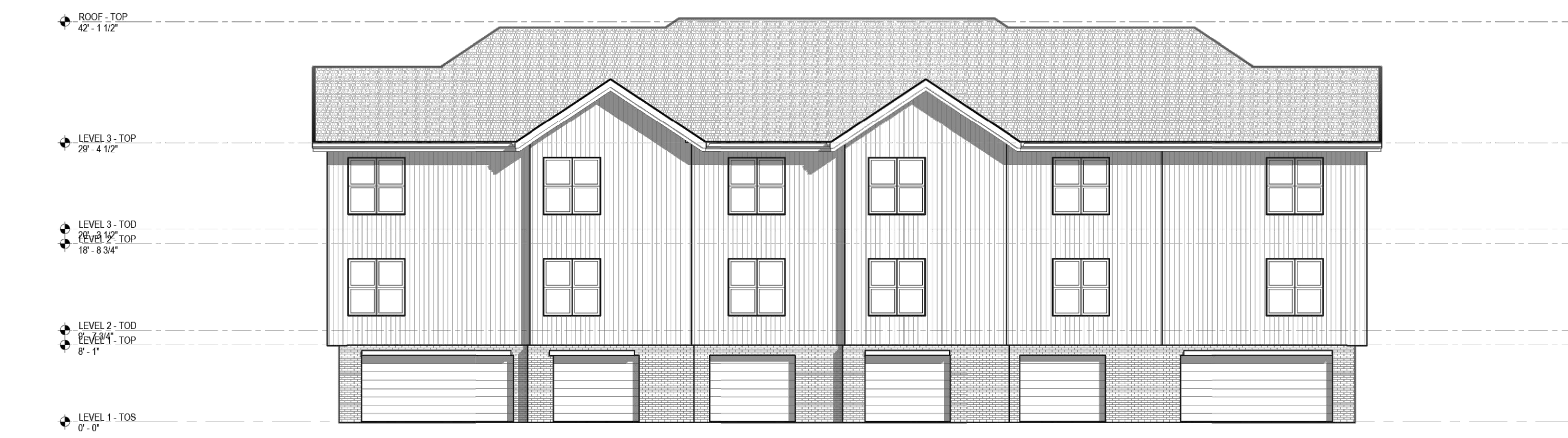
1 BUILDING TYPE II - FRONT ELEVATION 1/8" = 1'-0"
