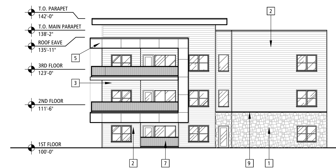
BUILDING 'B' SOUTH ELEVATION 1/16" = 1'-0"
