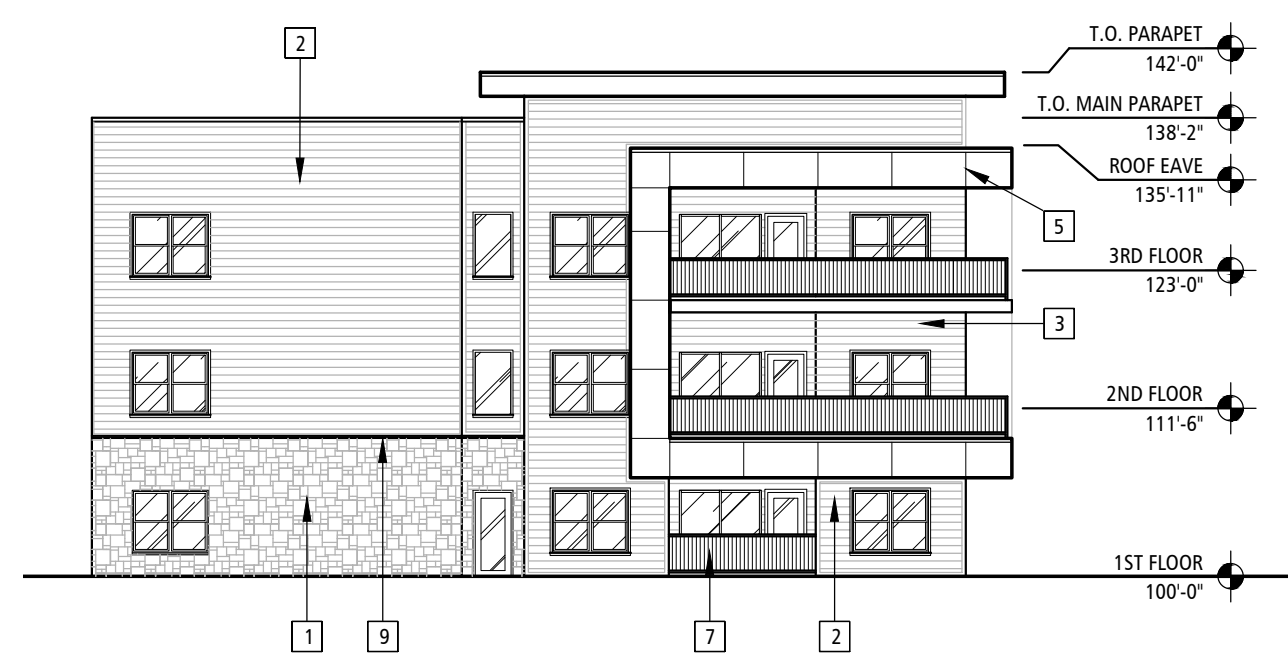
BUILDING 'B' NORTH ELEVATION 1/16" = 1'-0"
