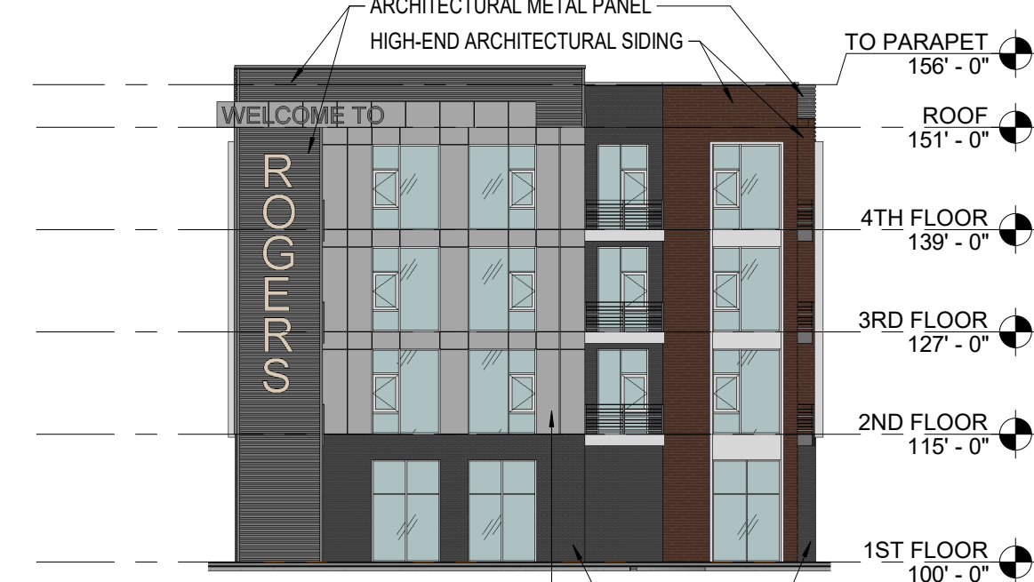
3 BUILDING 1 NORTH ELEVATION 1" = 20'-0"
