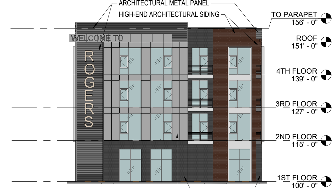
3 BUILDING 1 NORTH ELEVATION 1" = 20'-0"
